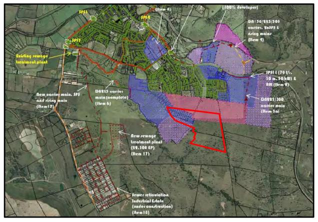
Figure 3 Extract from MSC Developer Servicing Plan – Sewer
